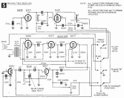
recheck wiring, particularly looking for solder shorts. A bad tube could also cause trouble.
