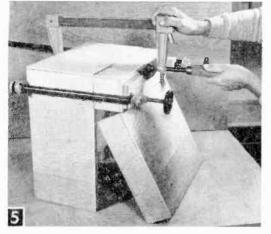
Top is sliced off changer compartment box, then glued back on again.
