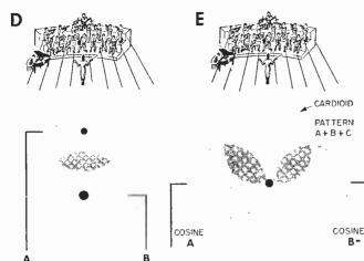
Longitudinal Method: o m n i - d i r e c tional mikes separate sound by time delay.
