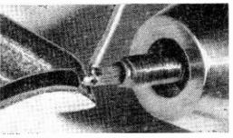
• A drill's chuck can double as that extra hand that's needed to hold small lugs, jacks, plugs, and other parts while you solder wires to them. Soldering is a lot easier and there's no chance of painfully burning your fingers on hot parts by trying to hand-hold them. You can use an ordinary hand drill for the purpose or an electric drill—either does the job nicely.—J.A.C.
