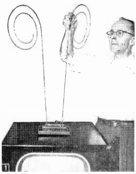
Each arm of this indoor television antenna can be rotated to bring the coiled sections in the best position for station reception.
