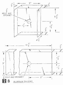
flat pieces of aluminum stock (see Fig. 2B). Scribe the flat pieces of aluminum along the sides to be bent, bend the aluminum and drill and fit with rubber grommets two  $\frac{1}{2}$ -in. holes as shown. These dividers are then fastened in place under the chassis with machine screws and nuts as shown in Figs. 2A (dotted lines) and 3.
