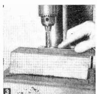
By tipping the drill press table the two holes drilled for the ends of the arms are given a 5° slant or you can hand drill by shimming up one end of the piece to get the right slant.
