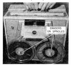
• If you ever need to carry your tape recorder in a vertical position with the tape spools still on the spindles, place a slipon pencil eraser over each spindle. This STORE IN SPOOL HOLES ."
