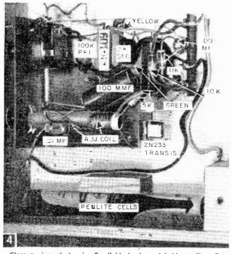
Closeap view of chassis. Small block of wood holds penlite cells in position. Four-lug tie-str/p simplifies mounting small components. Chassis is secured in box with a pair of 3-48 *fh* machine screws.
