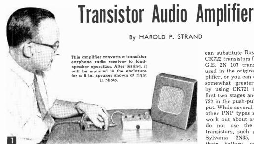
RANSISTOR experimenters who have built a radio for earphone reception soon find that they would like an amplifier to which the radio can be connected for loudspeaker operation. The amplifier shown here (Fig. 1) was designed especially for this purpose and will provide excellent volume with a 6 in. or larger speaker having a 3-4 ohm voice coil. The total cost of building the amplifier will be around \$18.00, including \$8.85 for the coupling transformers.
