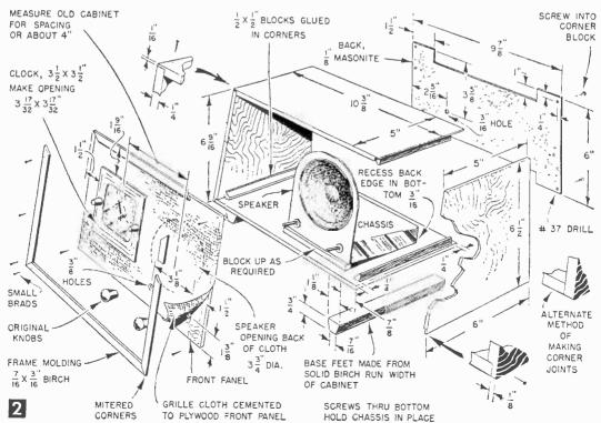
removed. The two wires connecting the radio to the clock line and the control switch are cut close to the terminals with diagonal pliers. To remove the receiver chassis, first pull off the knobs at the front and then remove the bottom screws.
