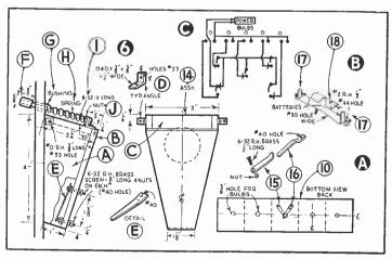
boxes and fit the contacts in place (Part E). Check these before mounting to see that they close under the weight of a single marble. Turn the handles (Part F in Fig. 6) from brass rod which has been cut to length, drilled and tapped for the 8-32 screw.
