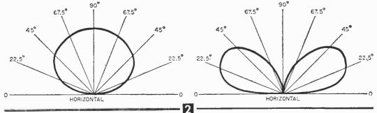
VERTICAL RADIATION PATTERN SIMILAR TO THAT OF TYPICAL HORIZONTAL DIPOLE. NOTE THAT MOST OF ENERGY IS RADIATED UPWARDS WHERE IT IS USE-LESS FOR LONG-RANGE COMMUNICATION. RADIAL DISTANCE IS PROPORTIONAL TO RADIATED FIELD STRENGTH. VERTICAL RADIATION PATTERN SIMILAR TO THAT OF PROPERLY INSTALLED "CLOSET-TANK FLOAT SPE-CIAL" ANTENNA. NOTICE THAT CONSIDERABLY MORE ENERGY IS RADIATED AT ANGLES BELOW 45° WHICH ARE THOSE MOST SIGNIFICANT FOR LONG RANGE COMMUNICATION.
