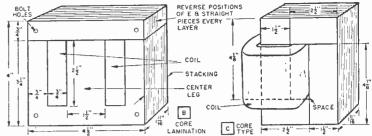
Core laminations (A) 1-piece shell lamination salvaged fram used radio power transformer. (B) E-type laminations (C) Core-type lamination made by alternating straight strips of silicon transformer steel. Transformers built on this core will require larger mounting box. (D) Coil winding form.
