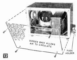
Back side of booster assembly. Voltmeter is set off center to clear transformer. Back screen allows air to circulate around transformer. Note fuse holder at right lower corner.
