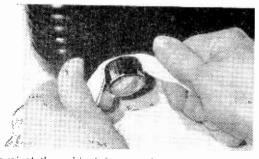
against the cabinet front with your thumb tips, at the same time pulling firmly at the cloth. The knob should work free without damage to cabinet or knob.—FRANK A. JAVOR.
