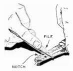
• A small notch filed into the bottom of a soldering gun's tip near the end makes it easier to hold the gun steady when soldering wires. The notch hooks over the wire connection and is especially handy for electronic builders and hobbyists with
