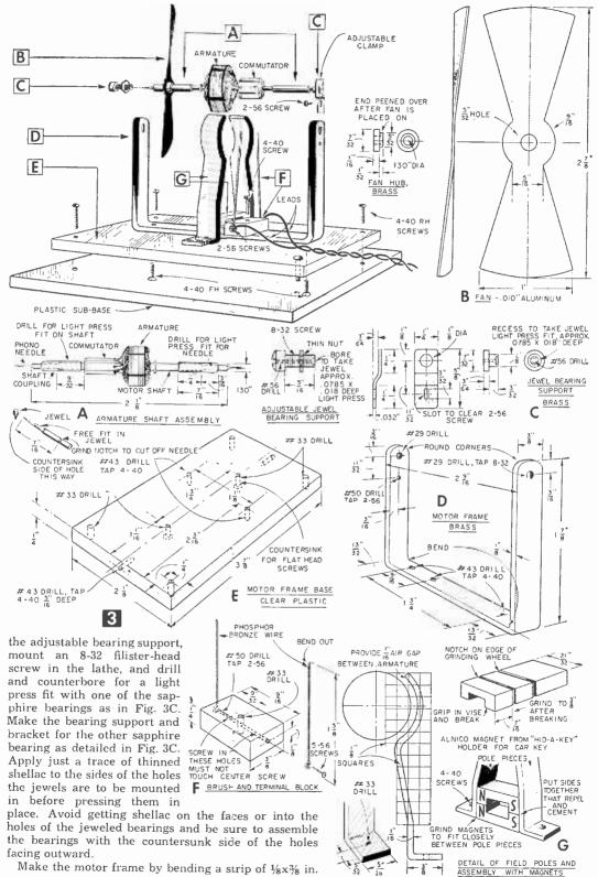
Make the motor frame by bending a strip of  $\frac{1}{8}x\frac{3}{8}$  in.
