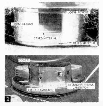
heads (See Fig. 1). A nylon brush on a typewriter eraser stick is an excellent tool for removing loose residue from the head structures. Loosen caked material with a lint-free rag moistened with rubbing alcohol or carbon tetrachloride wrapped around a wooden or plastic toothpick. Remove excess liquid with another clean rag.
