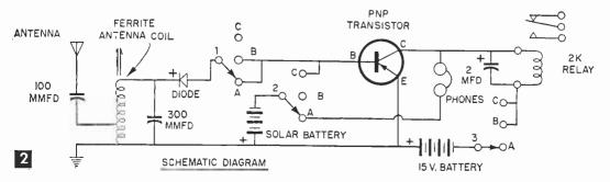
hearing-aid battery into the amplifier circuit. With a suitable antenna and ground attached to terminals the Transistorlab will now demonstrate how energy radiated by more powerful or nearby local stations can be made to operate other electrical circuits.
