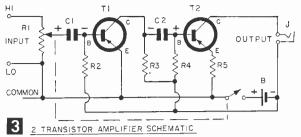
with a 2000-ohm earphone connected was 51 decibels. In terms of voltage gain, that's 320; the signal into the amplifier is magnified 320 times! To construct the amplifier (Fig. 1), cut and drill a piece of the miniature perforated Bakelite circuit board (see Materials List) as shown in Fig. 2. Make a matching set of holes for the phone jack and volume control in one half of the plastic case by making pilot holes with a heated ice pick and then reaming holes out to size with a taper reamer.
