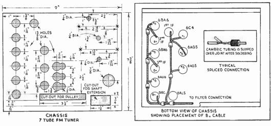
line cord), filament leads, B plus cable, ground connection bus (tinned #14 copper wire), RF coils (as shown in photo), and then the various resistors and capacitors, in that order. Make RF coils as shown in coil winding drawing; you may find that a very slight stretching or squeezing of the coils is necessary to obtain good alignment and tracking.
