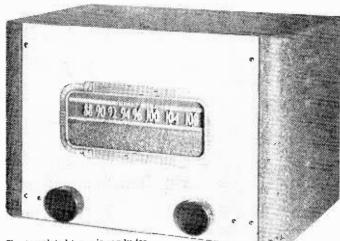
The completed tuner is ready for connection to an audio amplifier or phono jack on console radio.
