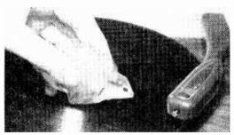
• If the grooves of your hi-fi phonograph records are filled with dust, here's how to remove it the harmless electrostatic way: Take a piece of Saran plastic wrap and crumple it in your fingers while holding it about an inch above the surface of the revolving platter. The static electricity produced by crumpling the plastic will attract the dust particles and hold them. If you watch very closely, you'll actually be able to see them jump from the platter to the charged wad of plastic.—J.A.C.
