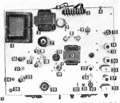
Power Transformer; 2) Filter Choke; 3) VR150 Voltage Regulator; 4) Line Card;
