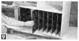
Masonite panels make good record storage dividers. Note narrower compartment in center.
