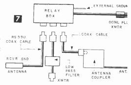
the octal plug, the other going to one side of the 110-v line. Connect the other side of the 110-v line to terminal 4 of the octal plug. Terminals 2 and 4 were chosen for the sake of convenience Any others can be used as long as the corresponding plug-socket terminals are used.
