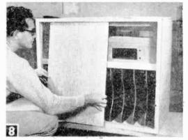
Deeper groove in top front-frame member allows sliding doors to be inserted.
