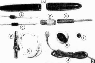
Component layout-A. Pen cap and barrel. B. Diode detector. C. Ceramic fixed capacitor. D. Coil. E. Tuning slug and screw. F. Small alligator clip. G. Antenna lead. H. Earphone. I. Tuner knob. J. Earphone Cord.
