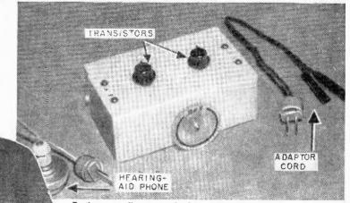
Testing an ordinary standard size magnetic earphone for use as a microphone with the transistor amplifier. Photo above shows how transistors are placed on outside top of case.
