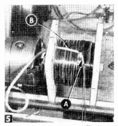
Bringing out loop tap at 247th turn. Slip sleeving over loop and separate lead from rest of windings with electrical tape, top and bottom. Continue winding over tap loops.
