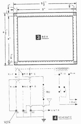
the coaxial cable directly to the relay posts (R1-C or R1-A). This will reduce the flexibility of the set-up, however, and should only be considered if absolutely necessary.
