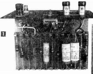
A compact and efficient unit designed for continuous service—a transistorized capacitor relay, front-panel and underchassis views.
