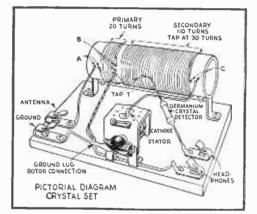
set, place taps every 10 to 15 turns while winding the secondary winding. But don't place any taps on the secondary before the first 30 turns.
