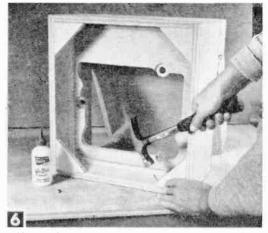
Glue blocks (not shown in Fig. 2) can be added to increase rigidity. Note cut-out for record changer.
