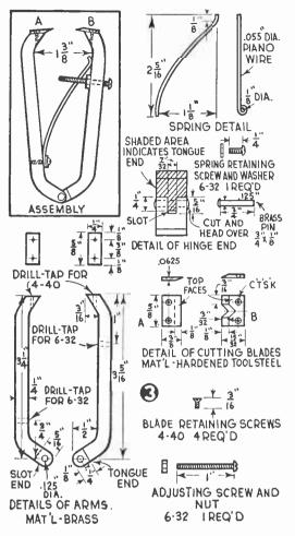
tersunk. With blades in a final finish condition, grind edges to a knife sharpness on a fine grit wheel. Harden blades with a Bunsen burner (Fig. 5) by heating to a cherry red, then plunging in cold water. Clean up one flat surface with
