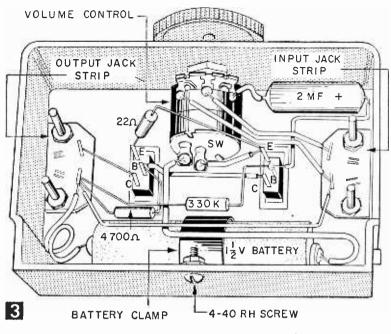
Using the Amplifier. Since all transistors are low impedance devices, this fact must be kept in mind when using the amplifier. A high impedance crystal microphone or phono pickup cannot be connected directly to the input. Nor can a crystal-type earphone be attached directly to the output of a transistor amplifier.
