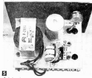
Back-of-panel, top view of unit showing transformer, coil, relay, sensitivity control and two transistors.
