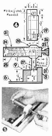
that's strong enough to throw marble against front panel but not so strong that marble will bounce off with considerable force when a miss is made. Next make the 2 metal angles (27) and assemble the unit together and to the slide.
