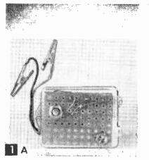
The basic two-transistor amplifier with clip-type input leads for general-purpose use (A). Volume control knob has been omitted in this photo to show simplified wiring more clearly. Piggy-back units are built on plastic case halves. In B, the basic amplifier is shown with an inexpensive flashlight battery power supply.
