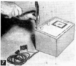
Fit birch frame molding to front to cover joints, set the brads and fill the holes. The pieces should be completely finished before fastening.
