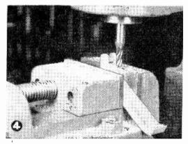
Fig. 4. Making hinge joint in a milling machine.
