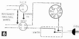
**Modification of Transmitter.** Many transmitters, such as the Heath AT-1, must be altered slightly to use this unit by replacing their SPST plate switch with a DPST switch. Reconnect the wires from the SPST switch within the transmitter to one side of the DPST switch and connect the other side of the DPST switch in series with the 110 ac drawn from the power supply plug and two prongs of the octal socket.
