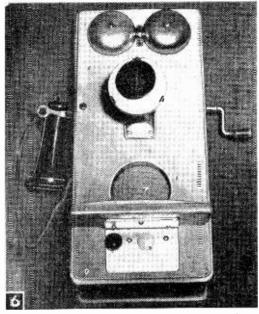
Refinished cabinet showing radio control knobs beneath writing shelf. Knobs of different colors were usea to distinguish between volume and tuning. Speaker g:ILe is 4 x 4 in. piece of aluminum fly screening taped to cabinet.
