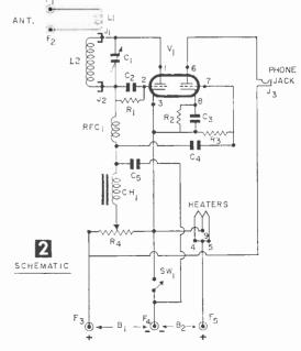
about  $\frac{3}{4}$ -in. from the top. The tuning capacitor (C1 in Fig. 2) is in the center of the sub-panel,  $1\frac{1}{2}$  in. from the top. Antenna jacks (F1 and F2) are on the right side,  $\frac{3}{4}$  in. apart, and the coil jacks (J1 and J2) are mounted 2 in. apart and  $\frac{1}{4}$  in. from the top edge of the panel. Screwfasten the front panel to the pine block.
