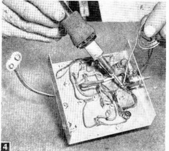
Flow the solder into the joints but avoid excessive use of solder which builds up a bulky joint.
