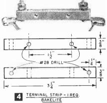
Completed terminal strip equipped with two Fahnestock clips and terminals for lead-in wire connections (Fig. 2).
