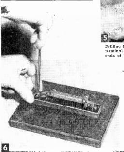
Roundhead wood screws fasten the Bakelite base piece to the wood base, through holes bored in the ends of the Bakelite.
