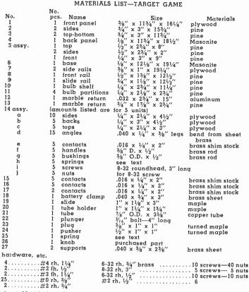
abcut 12  $\pm$ 2 rh,  $\frac{1}{\sqrt{2}}$  long for attaching back panel; small roll of bell wire, 5 flashlight bulbs, 2 flashlight dry cells, about ten glass marbles ( $\frac{3}{6}$ " D.), glue, brads. 1" finishing nails. Also 5 pilot light jewels—1 green, 2 red, 2 white (Allied Radio Co., 100 N. Western Äve., Chicago 80, Ill.) to fit  $\frac{1}{2}$ " hole.
